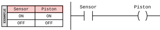
Fig. 1. Example code for a recycling plant in Ladder Logic, explained in detail in Section 2.
